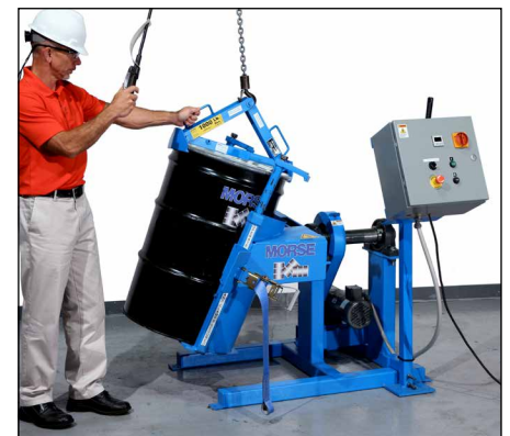
Load an upright drum into a 309 Series Drum Tumbler
