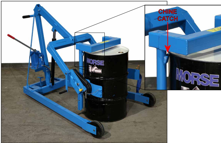
Approach upright drum with drum racker with two chine catches below the drum rim.
