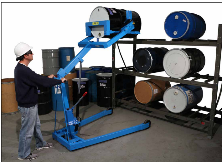
Rack a drum up to 72" (183 cm) high with a Morse Omni-Lift Drum Racker. Model 405 shown has hand pump drum lift and hand crank drum tilt control.
