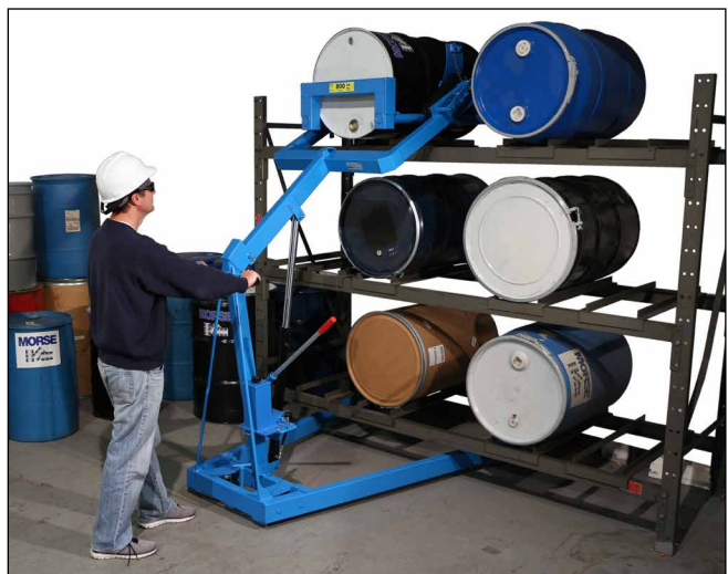
Place drum onto drum rack. Then back drum racker away. To remove a drum from a rack, simply reverse the procedure. Ensure that chine catches are engaged below drum rim and drum is secured with web strap and ratchet BEFORE tilting from horizontal position.
