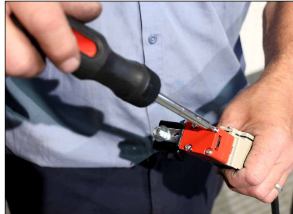
Ensure switch (item 5) is configured to receive key (item 2) with latch on left side of door.
