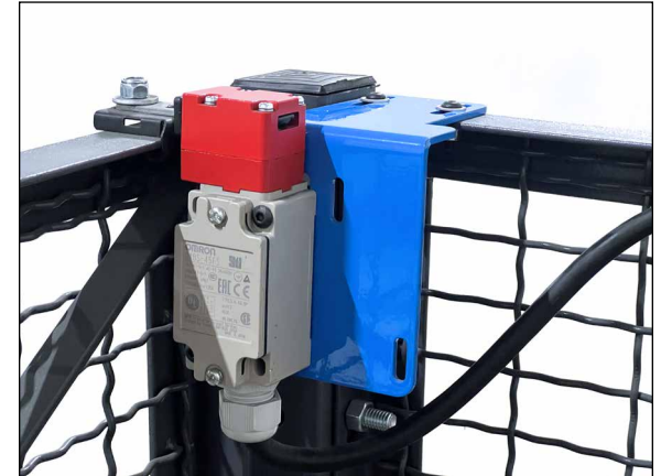
Close enclosure and verify that the key aligns properly with the switch. If key is not aligned properly, adjust accordingly. Key may be adjusted by loosening its screws and moving, then re-tightening screws. Use zip ties to retain cable from switch to control station.
