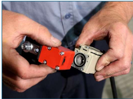
If necessary, reverse orientation of switch. . .
