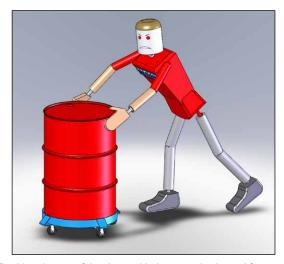
Pushing the top of the drum with the same horizontal force will result in a 73% load shift to the front wheels of the dolly. The dolly can become difficult to control and potentially hazardous - even tip over, especially if the dolly wheels hit an obstruction, a hole in the floor, or you descend a slope.
