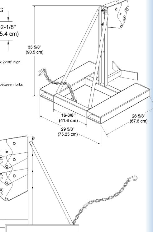
Mount Head with Jaws at 3 different positions in order to handle various height drums
