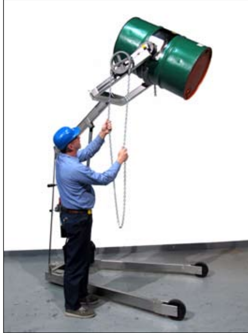
Turn drum 360° in either direction with pull chain and chain wheel. Models are also available with battery, electric or air power drum tilt (see chart at top of page 2).
