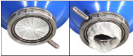
Iris Valve for controlling the flow of fine and coarse materials. Revolve the handle around the valve to open and close the flexible sleeve.
