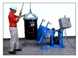
Load drum with hoist using appropriate drum lifting equipment, such as model <u>92 Below-Hook Drum Lifter</u>.
