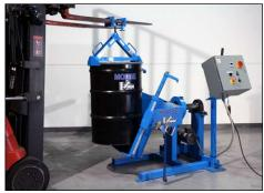
Load drum with forklift, using appropriate drum lifting equipment, such as Morse <u>model 284 Fork Hook</u> and model 92 Below-Hook Drum Lifter.
