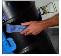
Place loop of web strap onto clevis
