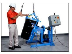
Guide the drum so that it tilts back and seats into the drum mixer as it is lowered.
