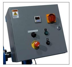
Morse NON-explosion proof AC Control Packages (sold separately) include control box with timer, start and stop buttons, variable speed control from 2 to 20 RPM, emergency stop button and lockable fused disconnect.
