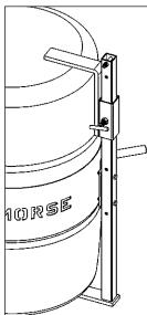
**Bracket Assembly** part # 4556-P Plastic drum being lifted with Bracket Assembly installed.
