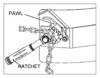
hold back the drum rotation. The chain lock on the bottom of the power arm can be used to prevent drum rotation. To do so, criss cross the chain and insert in each slot of the chain lock.
