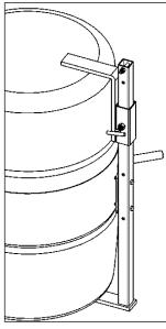
Figure 2.2 drum Plastic lifted with part number 4560M-P Top Rim Clamp Assembly installed.
