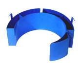
Diameter Adaptors for drums from 18.5" to 22" (47 to 55.9 cm) in diameter do not have hold-down brackets. They fit between the ribs of a steel drum. For plastic or fiber drum, use Diameter Adaptor in combination with the Bracket Assembly to prevent the drum from slipping lengthways through the drum holder.
