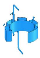
Diameter Adaptors for smaller drums from 14" to 17.5" in diameter are equipped with adjustable hold-down brackets to prevent your drum from slipping lengthways through the drum holder. Handle a drum up to 38" tall.
