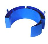
Diameter Adaptors for drums from 18.5" to 22" in diameter do not have hold-down brackets. They fit between the ribs of a steel drum. For plastic or fiber drum, use Diameter Adaptor in combination with the Bracket Assembly to prevent the drum from slipping lengthways through the drum holder.
