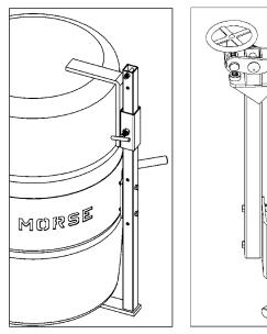
Figure 2.1 Plastic drum being lifted with part number 4556-P Bracket Assembly installed.
