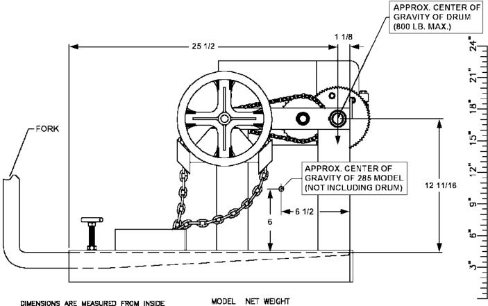
DIMENSIONS ARE MEASURED FROM INSIDE OF FORK TUBE END. THIS WILL GIVE A FIXED POINT TO WHICH LOST LOAD DATA CAN BE DETERMINED. (FORKS MUST BE TOUCHING THIS FORK TUBE END.)
