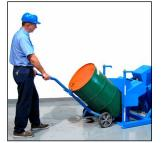
Load drum with drum truck
