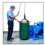
Load drum with hoist attachment
