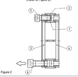
Prior to initiating the following removal procedure, check to ensure that no torque or thrust loads are acting on the Keyless Bushing, shaft or any mounted components.
