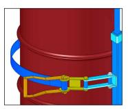
3. Drape the web strap across the face of the drum, and thread through slot in ratchet. Operate ratchet to tighten strap around drum.
