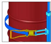
4. Operate ratchet to tighten strap around drum.
