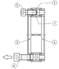
Prior to initiating the following removal procedure, check to ensure that no torque or thrust loads are acting on the Keyless Bushing, shaft or any mounted components.
