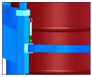
3. Drape the web strap across the face of the drum, place strap loop between clevis and secure with pin.
