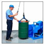
Load drum with hoist attachment
