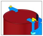
5. Turn the top clamps until they tighten against top of drum. Then remove hand crank BEFORE rotating drum.
