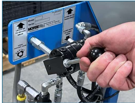
Start drum rotation by raising lever on left
