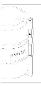
Figure 2.1 Plastic drum being lifted with part number 4556-P Bracket Assembly installed.
