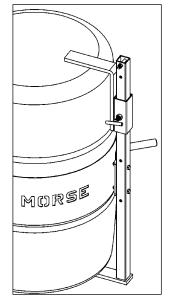
Figure 2.1 Plastic drum being lifted with part number 4556-P Bracket Assembly installed.
