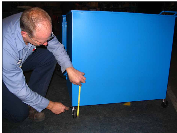
Step 9: Adjust the three casters so bottom of cage is approximately 4" off the floor. Do not lock in place just yet. Close enclosure and verify that the key aligns properly with the switch. If key is not aligned properly adjust casters accordingly. Key may also be adjusted by loosening its screws and moving (shown left). Once key is aligned properly, lock casters in place by tightening jam nut upward.
