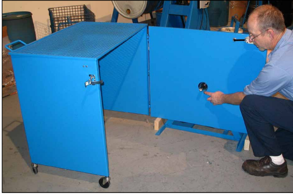
Step 6: Place the back panel of the enclosure onto the 2 x 4 spacers and against the frame of the tumbler. Center the hole with the shaft.
