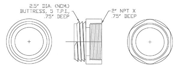
NOTE: BUTTRESS THREAD FITS 63mm OPENING OF MOST U.S. MADE PLASTIC DRUMS.
