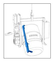
A 55-gallon (208 liter) plastic drum can be handled if the unit is equipped with the adjustable Bracket Assembly (Part # 4556-P). This bracket bolts onto the drum holder, and prevents a 55-gallon (208 liter) plastic drum from slipping lengthways.
